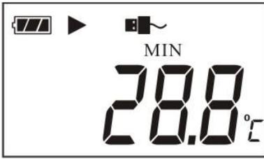
**Figure 14:** Minimum temperature recorder
